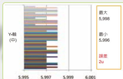
The machine maintained a repeatability of  $\pm 2 \mu\text{m}$  over 50 consecutive punches, showcasing precision comparable to premium Japanese and Swiss models.
