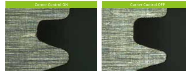
The unique corner control function ensures ultra-precise machining quality.
