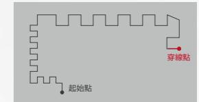
After a cutting interruption, threading resumes at the break point for immediate machining—no need to return to the start, reducing idle travel time.
