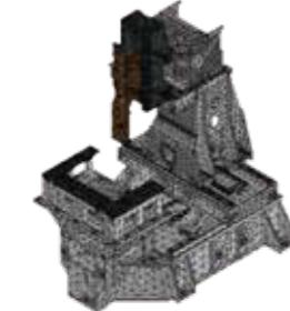
Utilizing FEA (Finite Element Analysis) to optimize the moving column structure, this design enhances rigidity and stability. The reinforced base and slideways ensure exceptional precision even during simultaneous XY-axis movement. Long-term machining performance is consistently outstanding.
