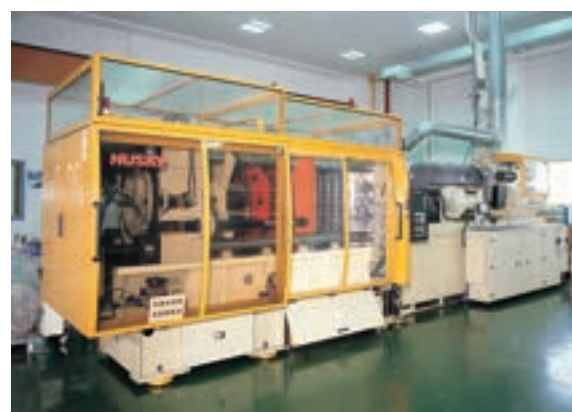
PET耐熱結晶瓶一瓶胚射出設備 High-Speed Preform Injection Machine
