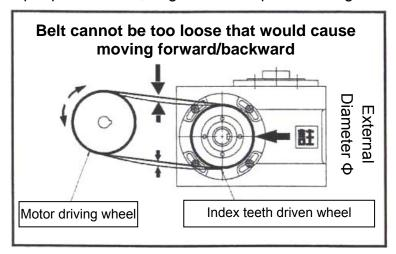
(4) The importance of belt, core and key: no loose is allowed between the belt wheel and input shaft core; otherwise, the belt wheel would move forward/backward that cause the inertia force: vibration and jerk, etc.
